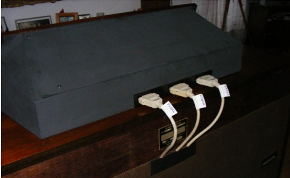
Fig. 3: My solution for connecting the controller box to the instrument. Every 25 pin connector carries the signals to and from on of 3 individual Orchestra Sections.
